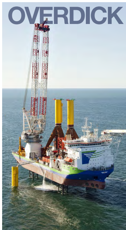
The North Sea jack-up vessel is designed for operations in water depths up to 50 m
