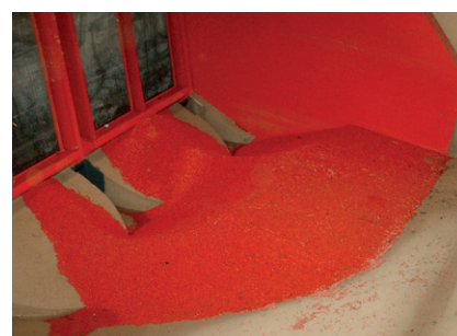
Sediment sluices under a power intake after a successful test (before and after flushing operation – 1:35 scale model).
