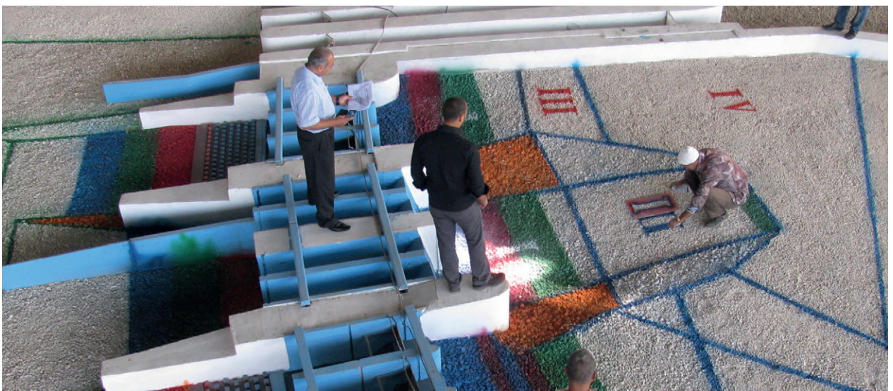
Physical model tests of scouring protection measures
