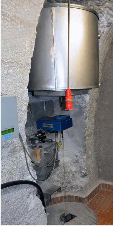
Pendulum in a concrete arch dam
