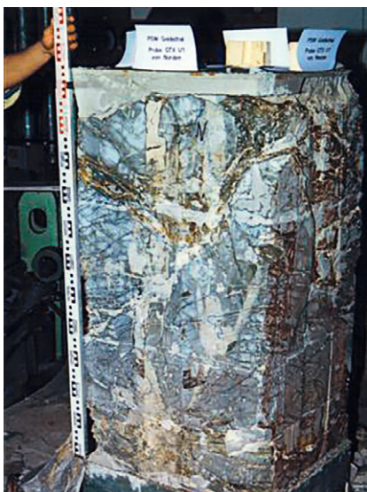
Specimen preparation for large-scale triaxial testing (Goldisthal, Germany)
